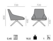
Frame Solid beech central swivel base with self-return system. Polished aluminum plate fixes the base to the seat. Base
